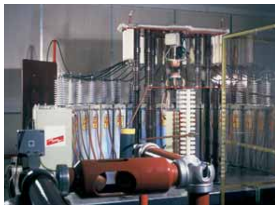
Fig. 9.16.1 Impulse current laboratory DEHN + SÖHNE – Max. lightning impulse current 200 kA, wave form 10/350 µs
